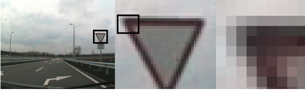
Fig. 4. Human color perception is a fuzzy process from a computer's point of view. While the first image clearly shows a red traffic sign for human eyes, one can see how color information changes by magnification.
